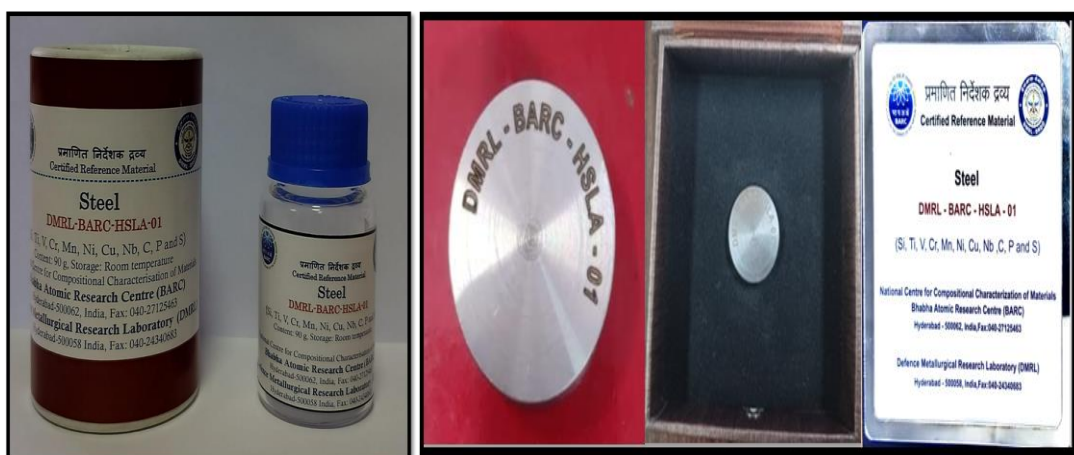
Chip and disk forms of HSLA steel CRM (DMRL-BARC-HSLA-01).
