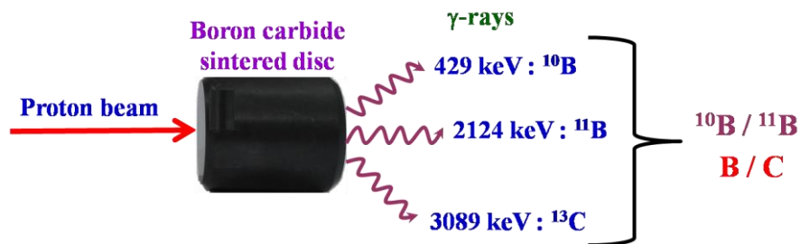
Figure 1: Schematic of PIGE method for determination of boron
